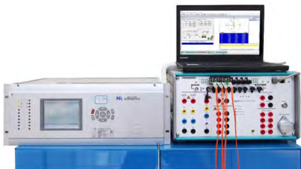
PW636i-F test digital protective relay (SMV+GOOSE)
