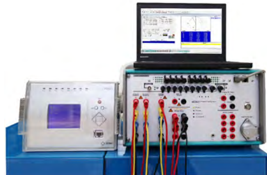
PW636i-F test traditional protective relay (Analog + Binary)
